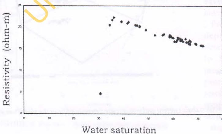
FIGURE 8: Resistivity - water saturation cross plot of reservoir: resistivity values tend to increase with decreasing water saturation.
