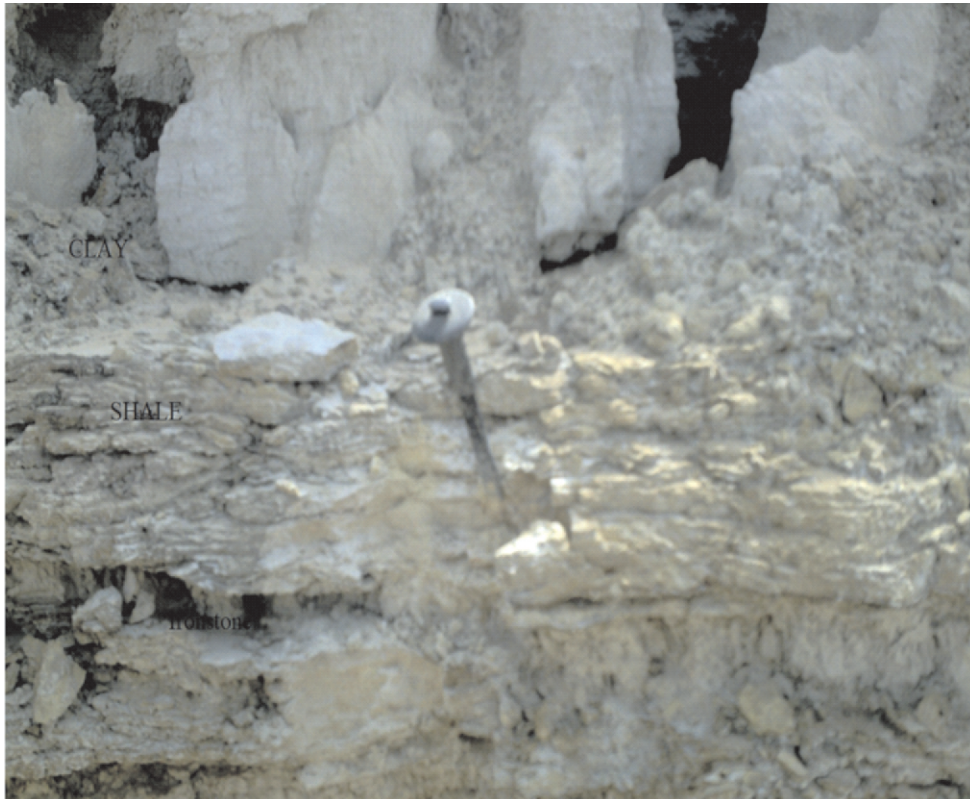
Fig3b. Field photograph of interbedded claystone, shale and ironstone at Ahoko- Latitude 8° 19.N and Longitude 6° 53' E Elevation of 82m
