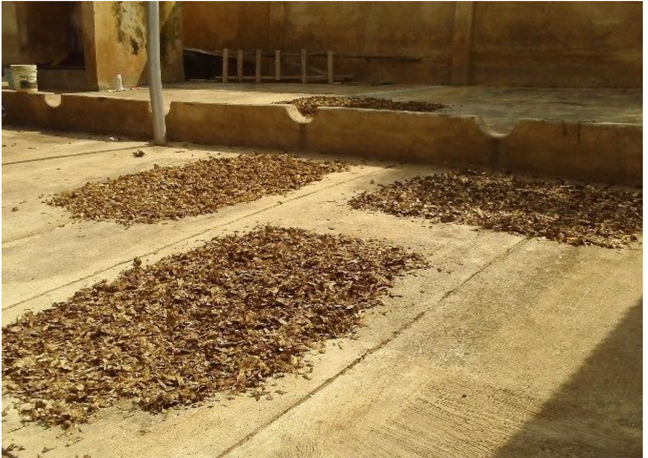
Plate 4: Fermented graded mixtures of OPS and CaP during sun curing
