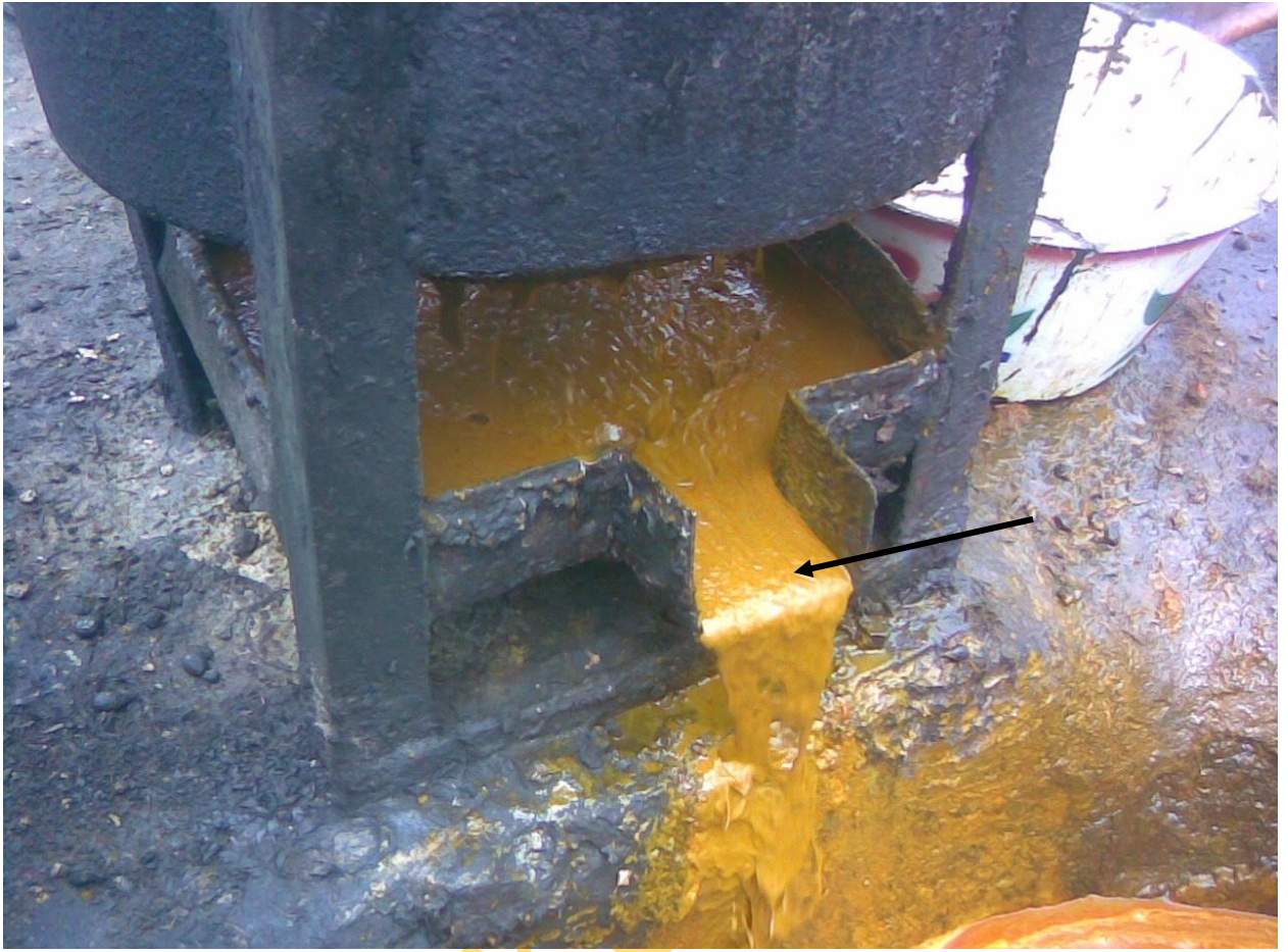
Plate 1: Clarified Oil palm slurry from a palm oil processing site at Mamu (Arrow is indicating slurry)
