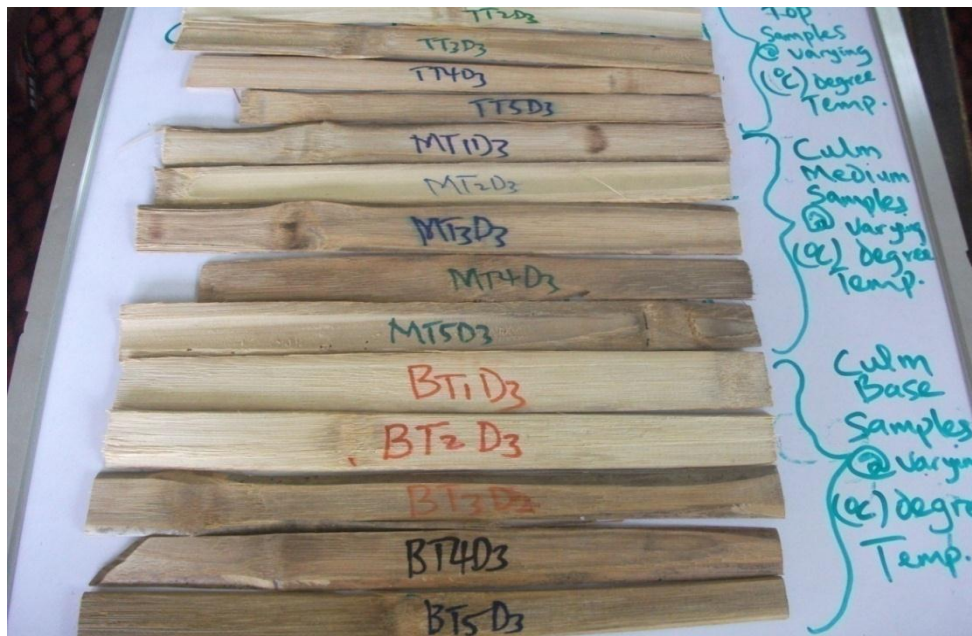
Plate 20: Colour variations in the thermal modification of Bambusa vulgaris
