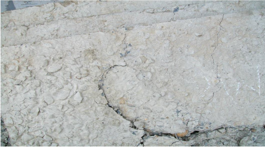
Plate 10: Crack pattern for waffle slab W5 Supported on 1 long side and 2 short sides
