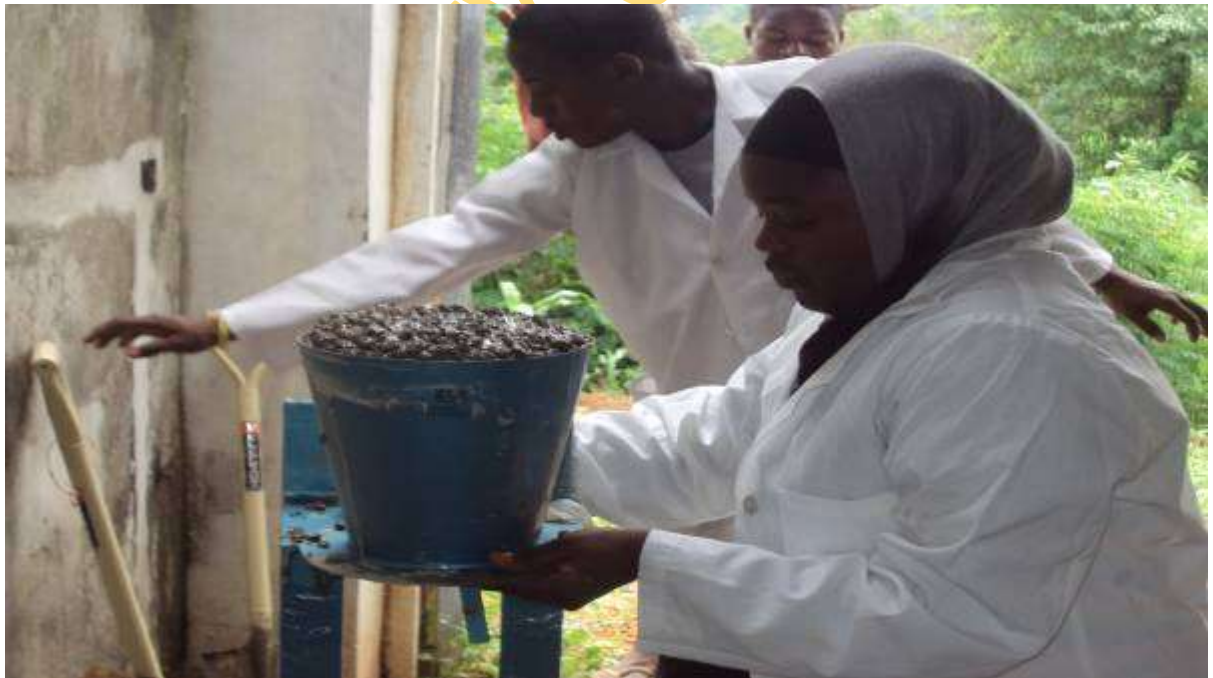
Plate 3.6a. The Compacting Factor Apparatus Ready for Use
