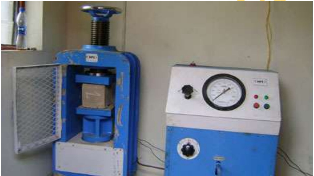
Plate 3.8. Cube in a Compression Machine Ready for Crushing
