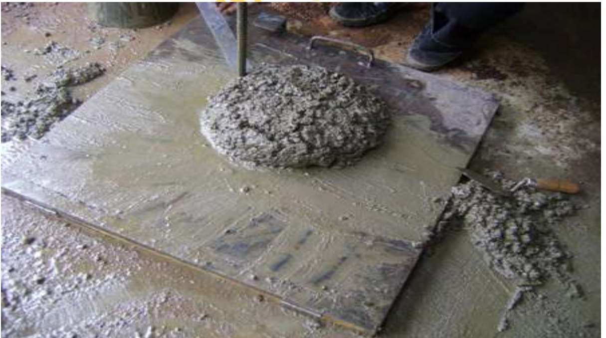
Plate 3.7a: Flow Table (Locally fabricated) Test in Progress
